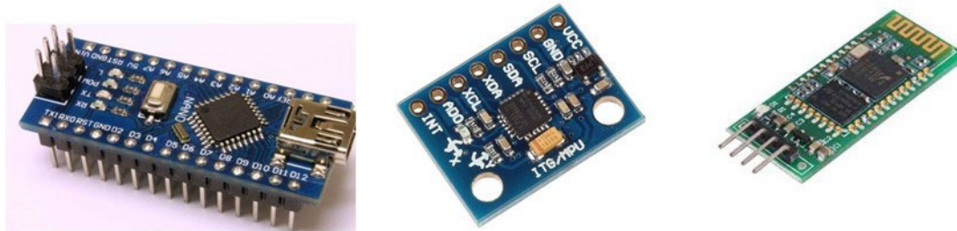
Figure 5: Sensors Package Used to Capture Ship Model's Motion.
