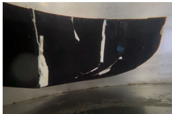
Figure 4: Crack Sample in Pool Environment.
