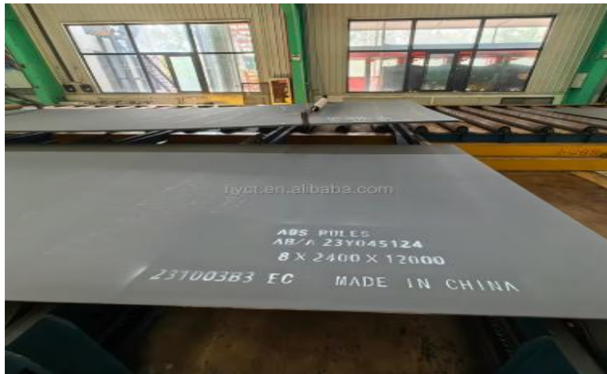
Figure 6: Steel Marking for plates and stiffeners
