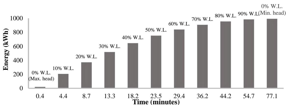
**Figure 5:** Power Output from the Filling Process
