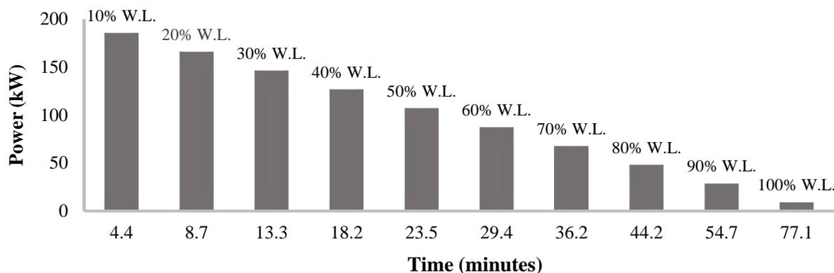
**Figure 4:** Generated Power Added During the Filling Process
