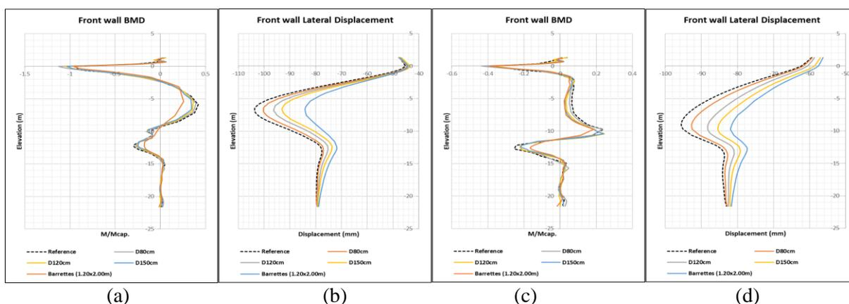
**Figure 9:** Impact of adjusting stiffness of piles: (a) Front wall BMD when sand fill is backfill, (b) lateral displacement when sand fill is backfill, (c) Front wall BMD when OC clay is backfill, (d) Lateral displacement when OC clay is backfill
