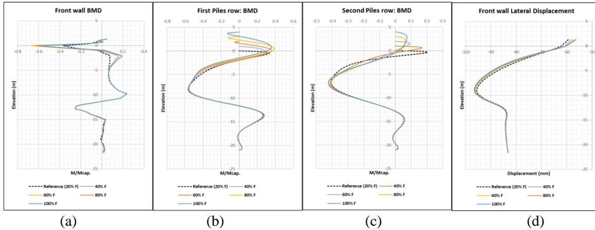
**Figure 14:** Impact of adjusting platform level when sand fill is backfill: (a) Front wall BMD, (b) 1st piles row BMD, (c) 2nd piles row BMD, (d) Lateral displacement
