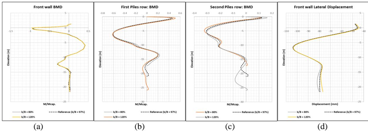
**Figure 12:** Impact of adjusting bearing level of piles when sand fill is backfill: (a) Front wall BMD, (b) 1st piles row BMD, (c) 2nd piles row BMD, (d) Lateral displacement
