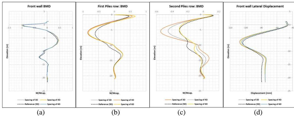
**Figure 10:** Impact of adjusting spacing of piles when sand fill is backfill: (a) Front wall BMD, (b) 1st piles row BMD, (c) 2nd piles row BMD, (d) Lateral displacement
