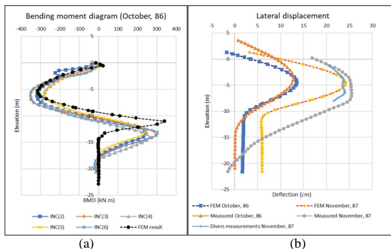
**Figure 3:** Front wall verification results: (a) Bening moments, (b) Lateral displacements
