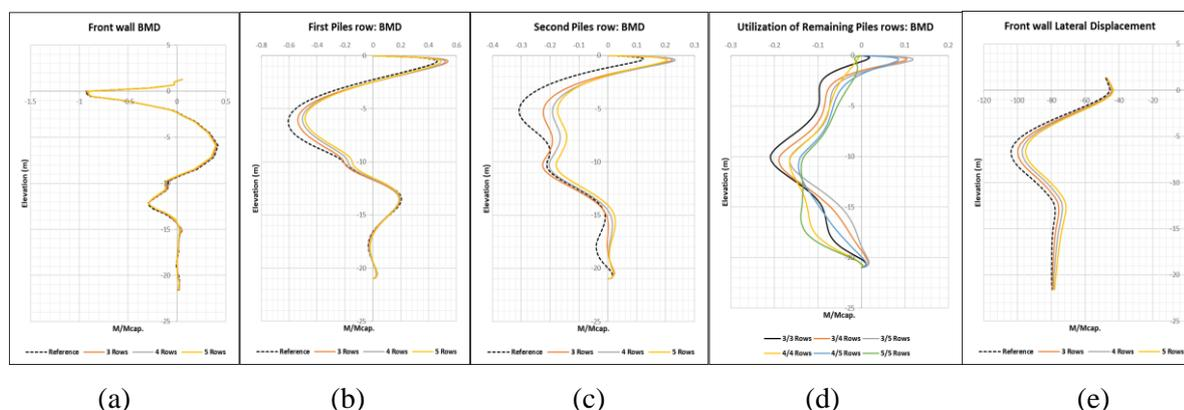
**Figure 7:** Impact of adjusting number of piles when sand fill is used as backfill soil: (a) Front wall BMD, (b) 1<sup>st</sup> piles row BMD, (c) 2<sup>nd</sup> piles row BMD, (d) utilization of the remaining piles, (e) system displacement
