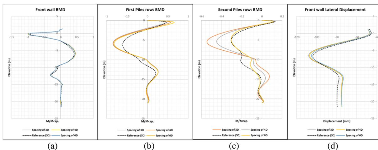
**Figure 10:** Impact of adjusting spacing of piles when sand fill is backfill: (a) Front wall BMD, (b) 1st piles row BMD, (c) 2nd piles row BMD, (d) Lateral displacement
