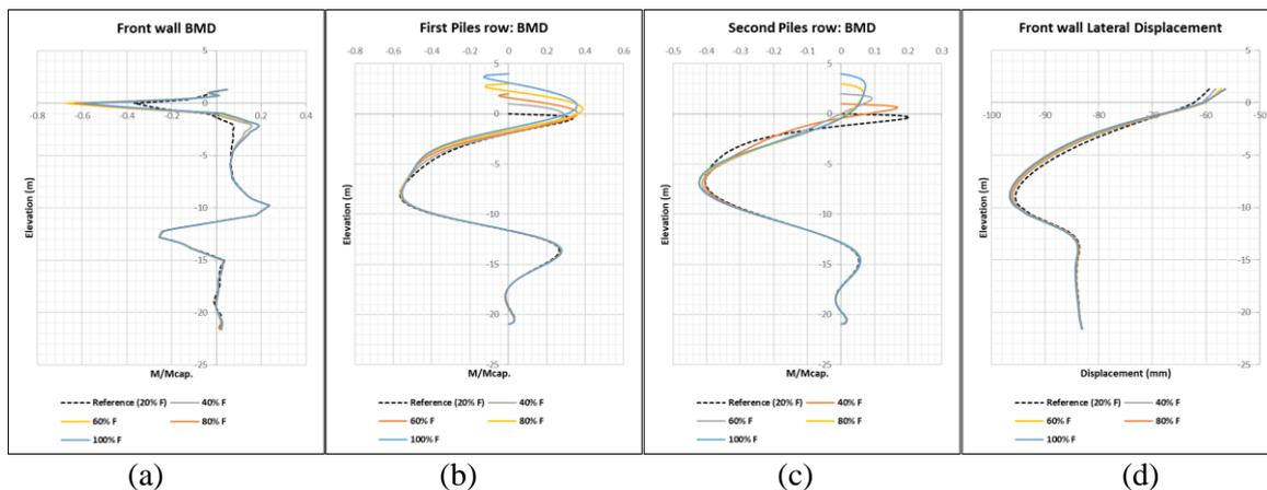
**Figure 15:** Impact of adjusting platform level when OC clay is backfill: (a) Front wall BMD, (b) 1st piles row BMD, (c) 2nd piles row BMD, (d) Lateral displacement
