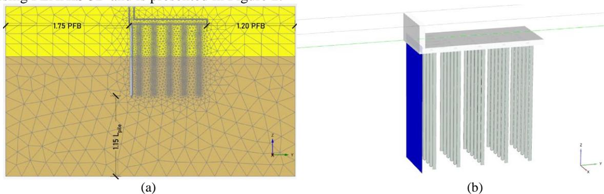
**Figure 2:** Numerical model: (a) Adopted meshing configuration, (b) perspective view of the model components
