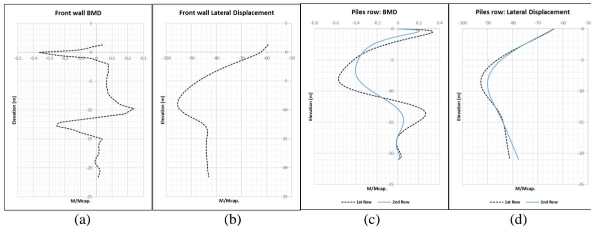
**Figure 6:** Straining actions of reference model 02: (a) Front wall BMD, (b) Front wall deflection, (c) Piles BMD, (d) Piles deflection
