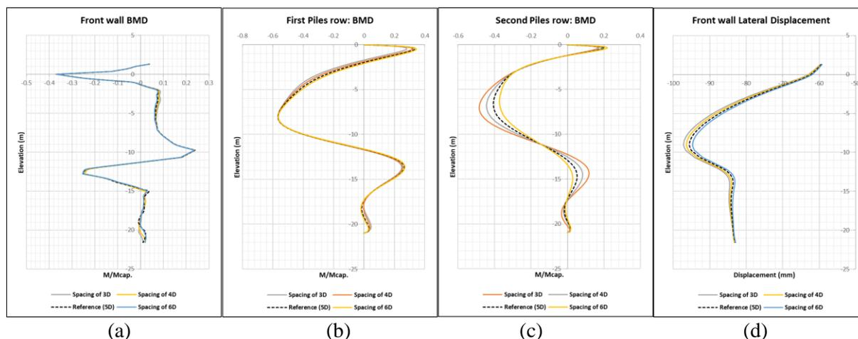
**Figure 11:** Impact of adjusting spacing of piles when OC clay is backfill: (a) Front wall BMD, (b) 1st piles row BMD, (c) 2nd piles row BMD, (d) Lateral displacement
