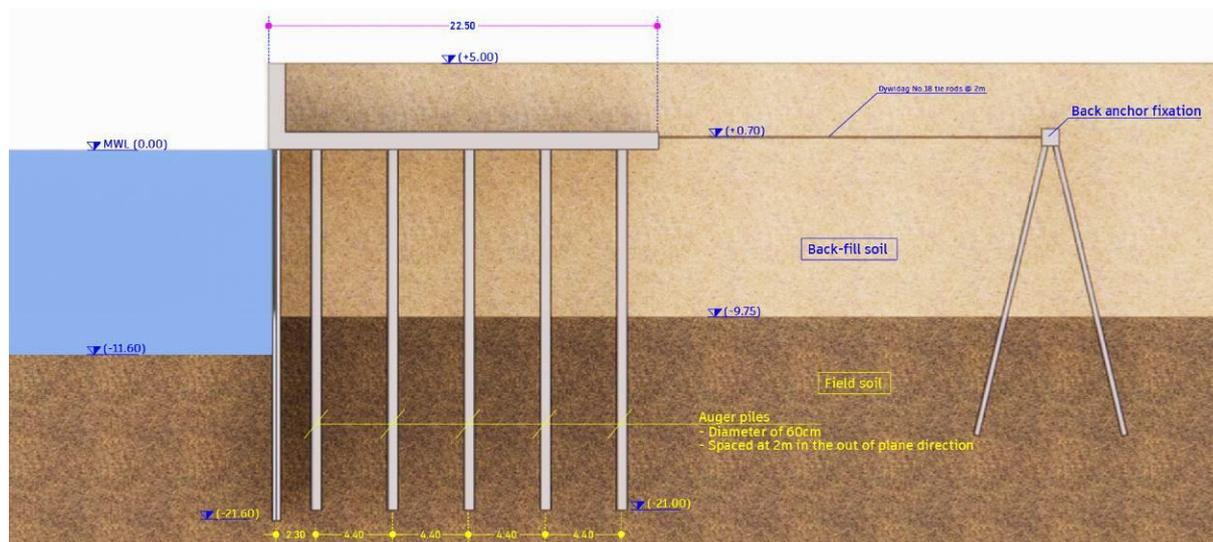
**Figure 1:** Cross-section of the measured quay wall
