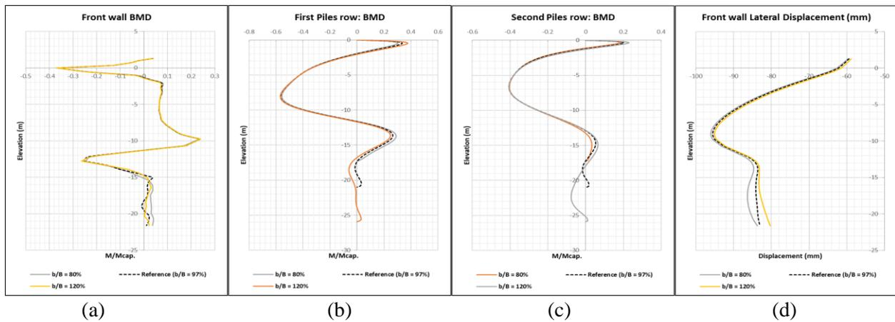
**Figure 13:** Impact of adjusting bearing level of piles when OC clay is backfill: (a) Front wall BMD, (b) 1st piles row BMD, (c) 2nd piles row BMD, (d) Lateral displacement
