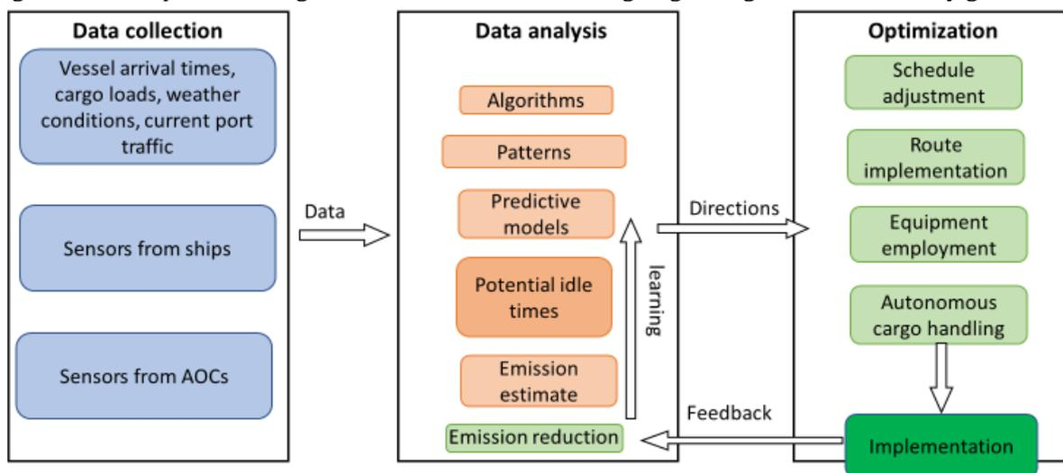
**Figure 1:** AI-Driven Emission Reduction in Port Operations Flowchart.
