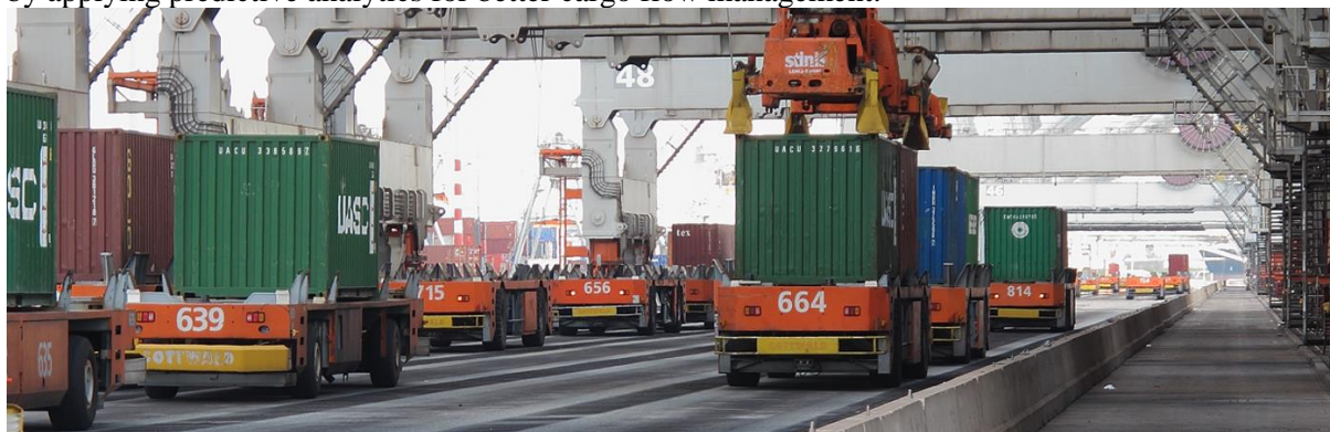
Figure 3: Automated Guided Vehicles handling shipping containers in Port of Rotterdam. Source: (“Sensors in the Rotterdam Container Terminal,” n.d.)
