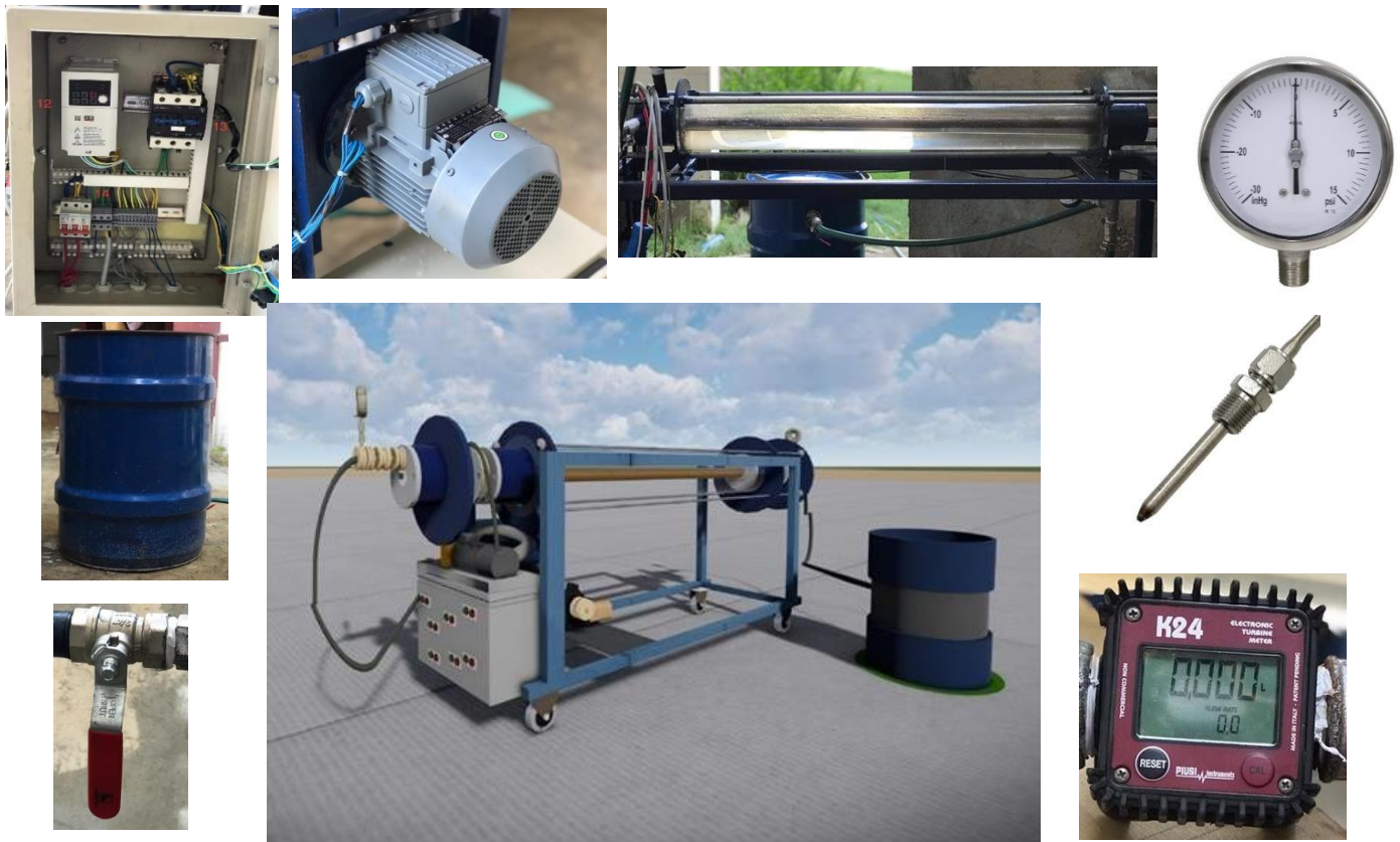
Figure (2) 3D representation of Heat Exchanger including the measuring equipments
