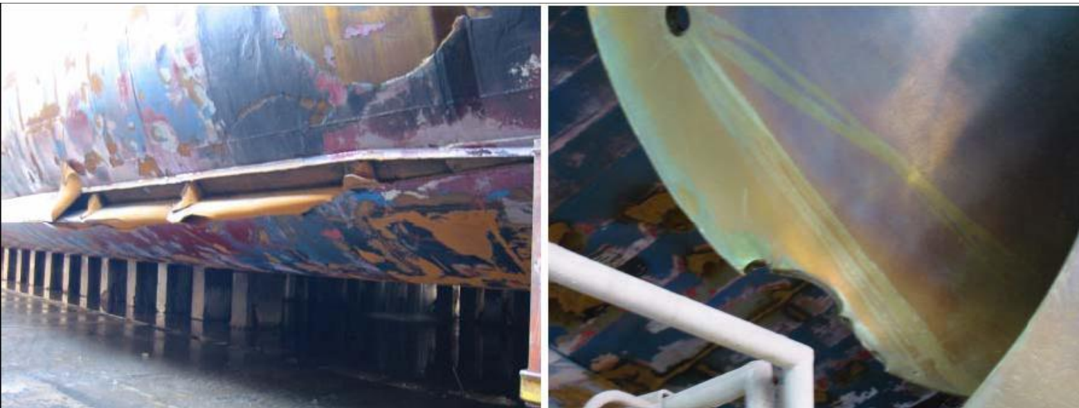
Figure 3-2: A Bilge Keel Rupture and Propeller Damage of Ship Number 100. Source: (Hänninen, 2003)
