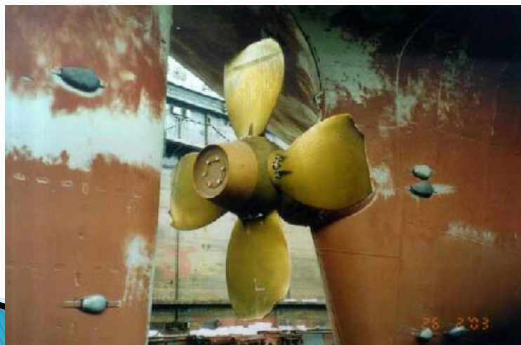
Figure 3-2: A Bilge Keel Rupture and Propeller Damage of Ship Number 100. Source: (Hänninen, 2003)
