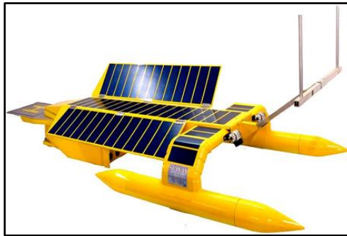
Fig. 10. Floating robot for cleaning plastic pollution
