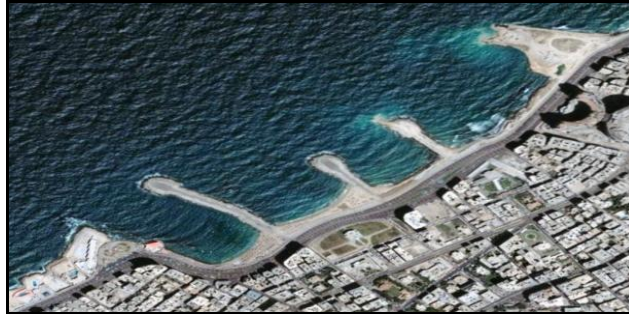
Figure 8: A satellite image for groins for Gelem Area, (Google Earth, 2009).
